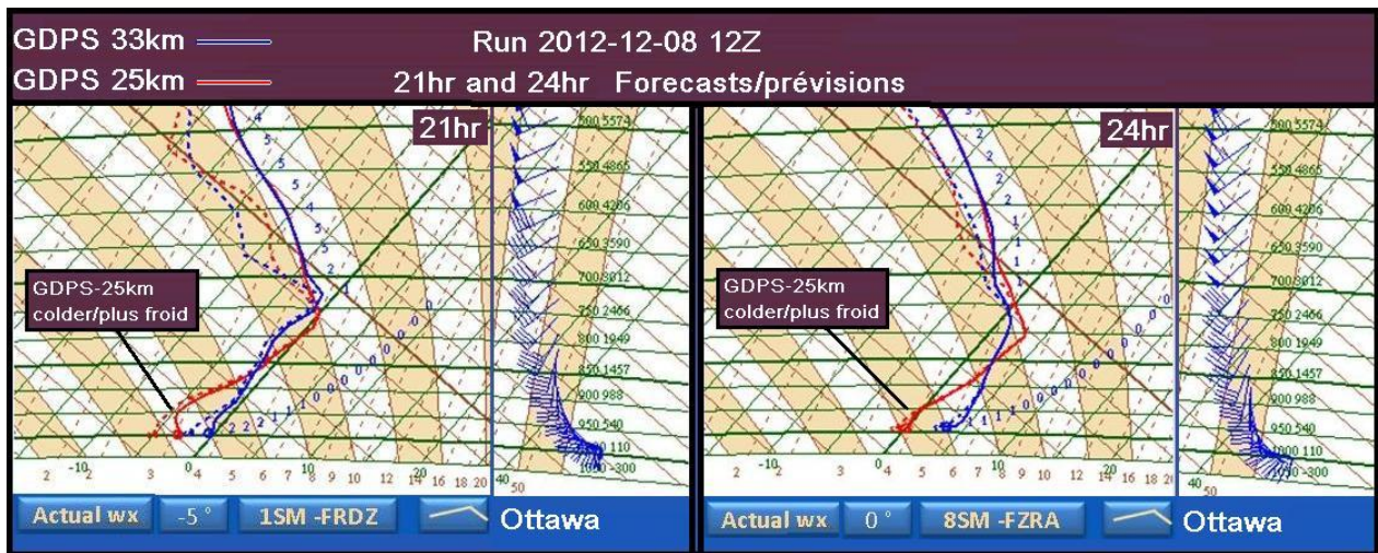
Figure 74: forecast tephigrams for Ottawa (YOW site), with lead-time of 21 (left) and 24 (right) hours, 18 December 1200 UTC forecast run; it shows the effect of the hysteretic effect in the planetary boundary layer (PBL) scheme introduced in GDPS-3.0.0. The GDPS-3.0.0 thermal profile is in red, that of the operational system in blue. Winds (blue wind barbs) are those of the operational system. The observed surface weather is in the blue ribbon at the bottom. This clearly shows how the inversion created by the warm air advection at mid-level and the near surface cold air advection is maintained the improved PBL scheme, producing a correct forecast of below freezing temperature and freezing rain.
