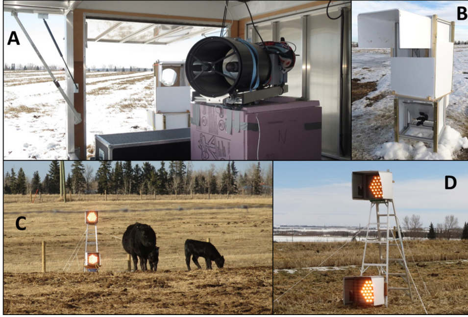
Fig. 1. Photographs of (A) the OP-FTIR unit inside a trailer (temporary box around the base insulates the aiming motor from cold); (B) the periscope; (C) the high-low reflector pair on the winter-feeding site; (D) reflectors on the winter-grazing site.
