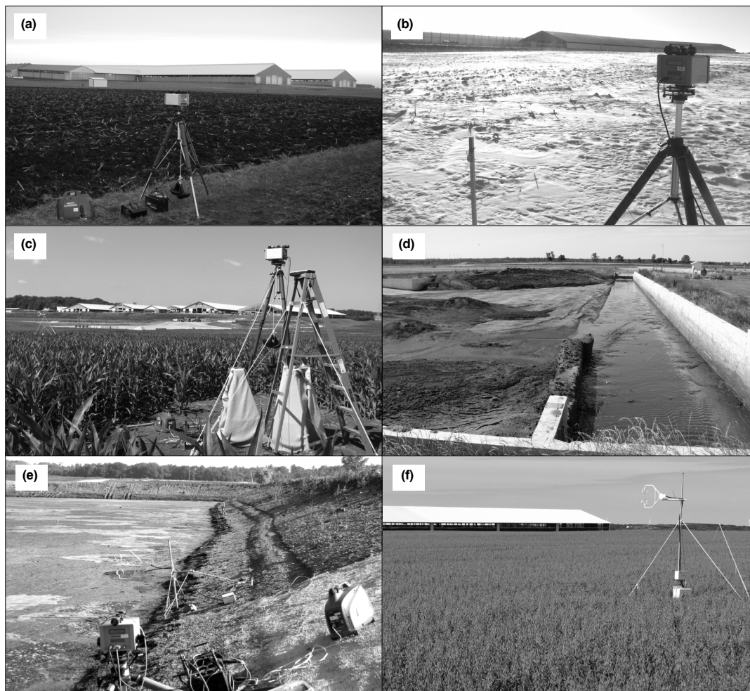
Figure 3. Photographs from the study: (a) laser measuring barn emissions at WI1-Fall, (b) measuring barn emissions at WI2-Winter, (c) measuring whole-farm emissions at WI3-Summer (laser on ladder to get above the corn), (d) sand separator, (e) laser and sonic anemometer at lagoon edge, and (f) sonic anemometer measuring ambient winds.
