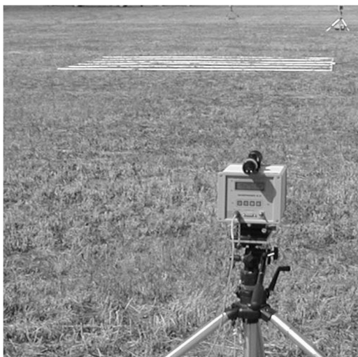
Figure 4. Line-averaging laser concentration detector and synthetic methane source at Ellerslie, Alberta [Flesch et al. , 2004].
