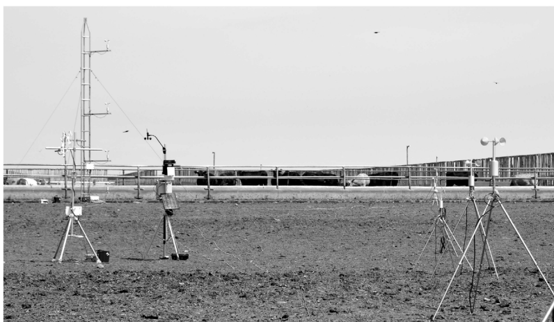
Fig. 3. View towards (roughly) the NNE across pen 37 (cup anemometer no. 1 out of view). The uppermost cup anemometer on the mast (“T4”) stood 5.08 m above ground. Note the sonic anemometer on the left-most tripod, matched in height to another on the 6 m tall, triangle-section mast.
