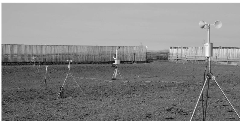
Fig. 2. View towards (roughly) the SSW across pen 37. Transect of seven cup anemometers all at η = 1.15 m above ground level (referred to in the text by number, no. 7 being the closest to camera). Anemometer no. 5 stood some 0.8 m below the mean level of the plot. Beyond the gate in the SW corner of the pen can be seen higher ground: the nearby berm of a feedlot reservoir, and (barely distinguishable) the foothills some 20–30 km distant.
