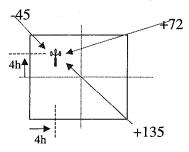
Figure 3: Anemometer at a "corner" position in the plot, and "corner flow" relative to that position, for which  $-45 \le \beta_r \le 135^\circ$ .
