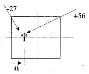
Figure 2: Anemometer at "side" position (x/h = -4, y/h = 0) in the plot, and ("reduced") wind directions  $\beta_r$  implying "corner flow" relative to that position, for which  $-90 \le \beta_r \le 90^o$ . Not to scale.
