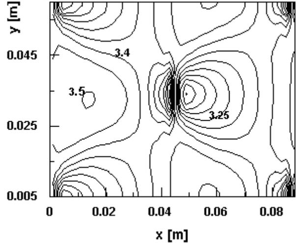
Figure 1. Contours of mean streamwise velocity  $\bar{u}$  [m/s] at  $z/H=1$  in the periodic Tombstone Canopy.
