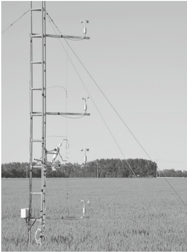
Fig. 1 View (telephoto lens) of the instruments and wheat crop, looking towards the south-west. Visible are the cup anemometers, the ultrasonic anemometer (at height z = 2.55 m above ground) and the open-path infra-red gas analyzer (LI-COR LI-7500). Also faintly visible are air lines, taped to a vertical wire and with their intakes coincident with anemometer heights. The LI-7000 analyzer is unseen within the crop. The distance to the north end of the taller trees (see right of photo) was 1.04 km and the bearing 240^\circ (i.e. 30^\circ south of west)
