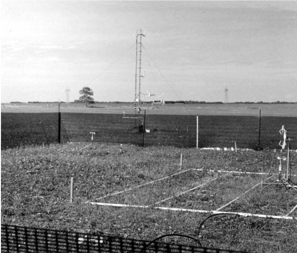
Figure 1. Windbreak experiment, Ellerslie, Alberta. A view to the south-west, showing several of the seven cup anemometers in-plot, a three-dimensional sonic, and a pvc manifold on ground (from which methane was released during gas dispersion trials described elsewhere).
