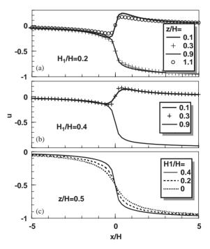
Fig. 1. Analytical solutions for the fractional velocity perturbation  $u = (1/k_r)\Delta U/U_0$  around a very porous windbreak, showing transects at several z/H as a function of gap depth  $\ell = H_1/H$ .
