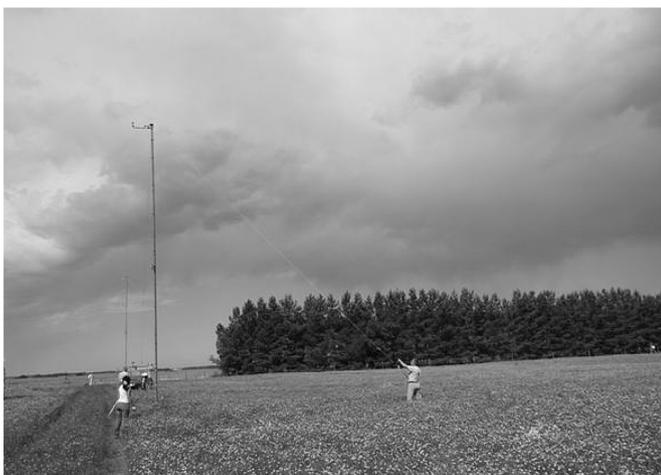
**Fig. 2.** View of the shelterbelt looking towards the WNW, roughly along the line of the reference (“unsheltered”) transect. The origin  $y/H = 0$  of the north–south axis is at the south (left) end of the shelterbelt, and the reference transect lies along  $y/H = -2.5$ .
